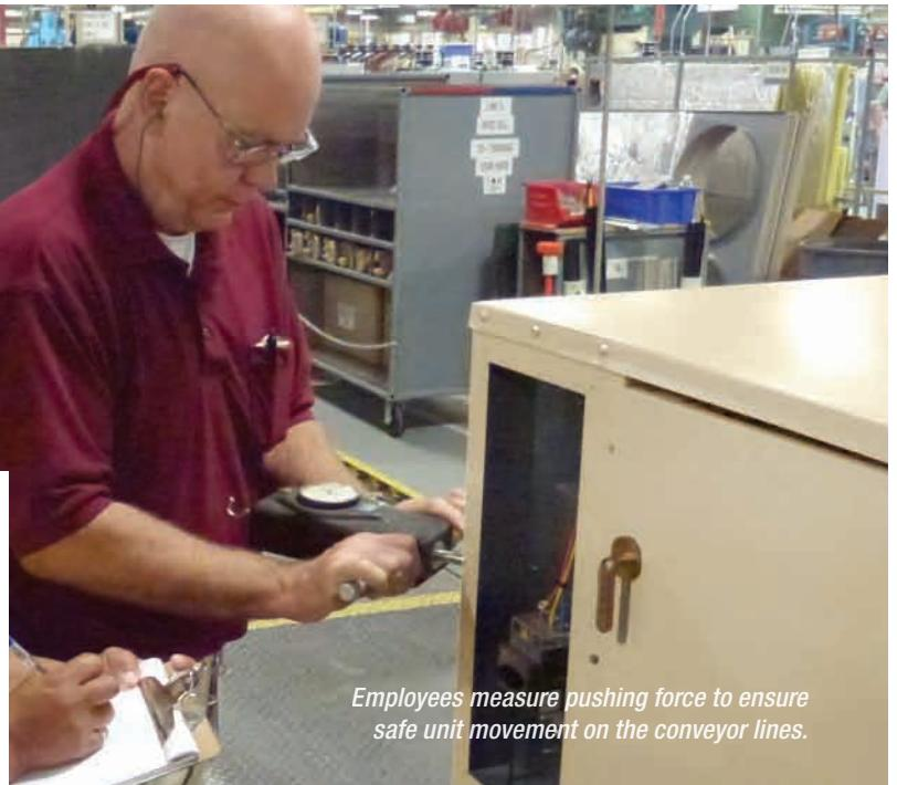
*Employees measure pushing force to ensure safe unit movement on the conveyor lines.*
